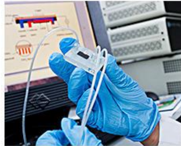
The innovative membraneless photocatalytic fuel cell can purify and use wastewater to generate power.
