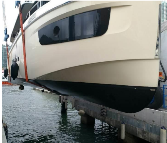
Photocatalytic antifouling paint
